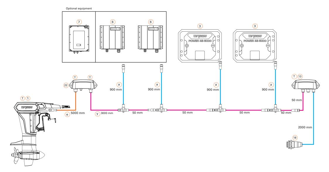
8 pin data cable5 pin data cable
